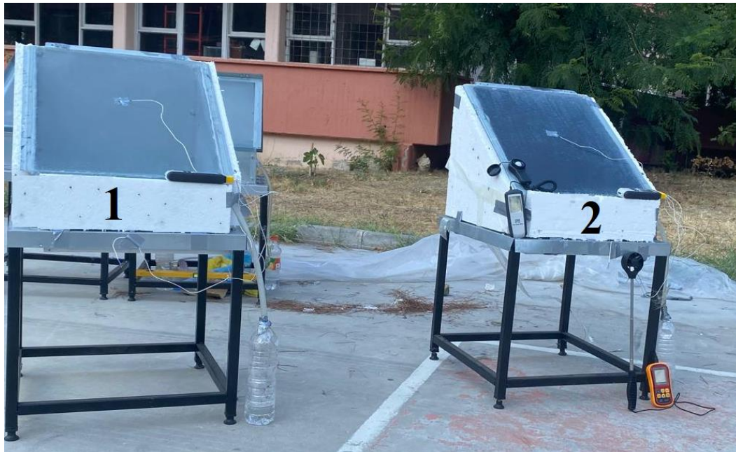
Figure 1. Experimental setups (Model number 1: unpainted, model number 2: interior surface matte black painted model)
